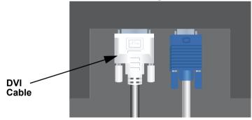
4. Connect the DVI connector at the other end of the signal cable to the DVI port located on the back of the graphics adapter. See picture below.
