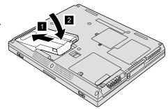
b) Slide the battery latch to the left to lock it.
