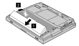
b) Slide the battery latch to lock it.
