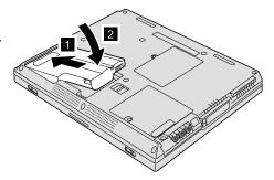
b) Slide the battery latch to lock it.
