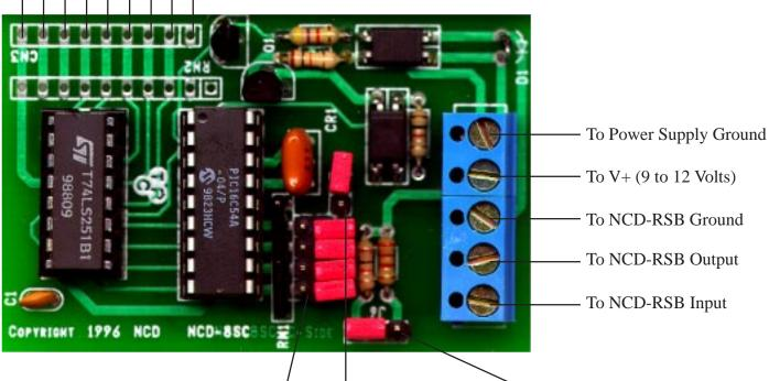
J1-J4 - Address Select. These jumpers define the device number of the 8SC, allowing 16 devices to coexist on a single serial line. See "NCD-110 Addressing" for details.
