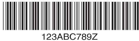
Figure 26. Code 3 of 9 Bar Code Example
