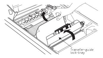
3 If you experience difficulty in removing the media, or if media isn't visible under the transfer-guide lock-tray, lift the green lever on the inner metal plate to check for jammed media under the metal plate. Remove the media.
