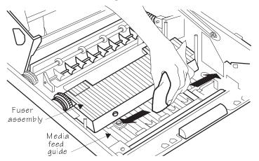
3 Using a dry, soft cloth, wipe the cleaned area to remove moisture.
