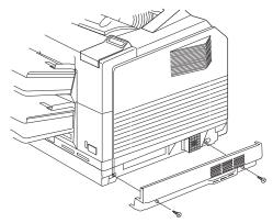
4 Remove the five screws on the metal tray assembly cover.
