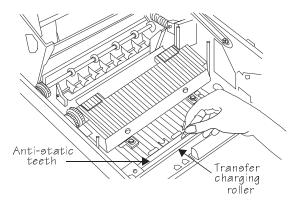
**Caution:** Be careful not to touch the transfer charging roller when cleaning the anti-static teeth. Finger oil, scratches, or other contaminants on the roller may reduce print quality.
