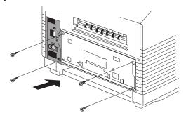
11 Replace the duplexing slot-cover, and reinstall the two screws that were holding it in place.
