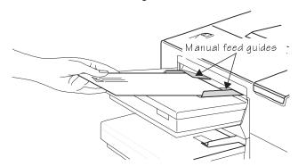
Because envelopes pass through heated rollers, the gummed area on the flap may seal. Open the flap immediately after it passes through the printer, before the seal cools. You may then reseal in the normal manner. The use of envelopes with emulsion-based glue avoids this problem.
