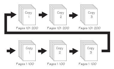
The maximum collation sequence is 100 sheets. Disk space of 10 MB is probably sufficient for most printing applications. The maximum
