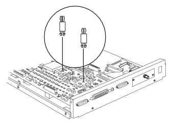
11 Snap the daughterboard on the two mini support posts and the two 48-pin connectors.
