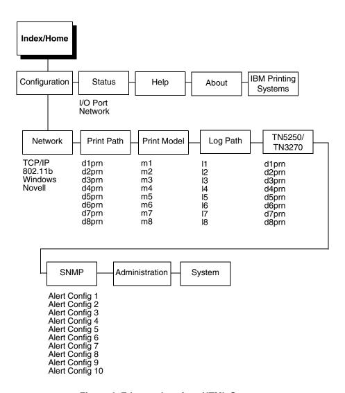
Figure 4. Ethernet Interface HTML Structure
