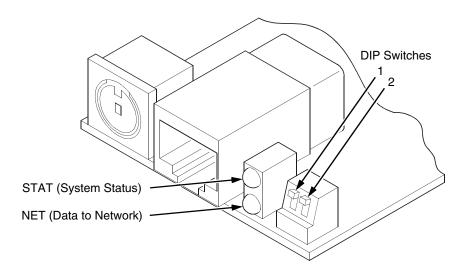
Figure 2. Status Indicator Lights and DIP Switches
