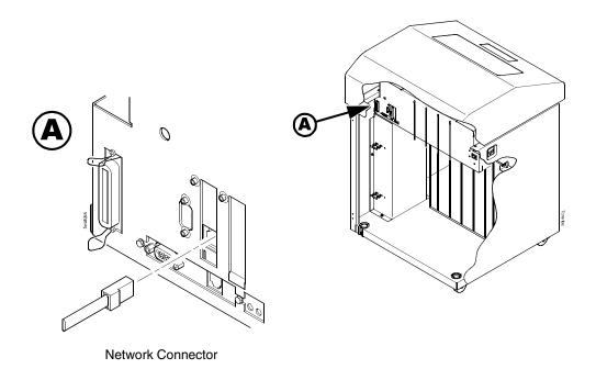
Figure 3. Interior View of the Cabinet Model Showing Network Interface Location and Setup
