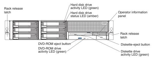
Rack release latches: Press these latches to release the server from the rack.
