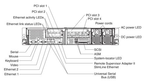
**Ethernet link status LEDs:** When these LEDs are lit, they indicate that there is an active link connection on the 10BASE-T, 100BASE-TX, or 1000BASE-TX interface for the Ethernet port.
