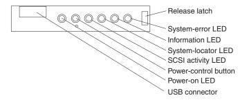
The following controls, LEDs, and connectors are on the operator information panel:
