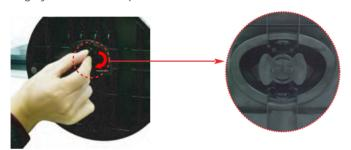
If you can't release the stand base even the locking rib is at a release position, Please push the indicated rib down and retry it.
