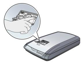
**Caution:** Don't turn off the scanner with a film strip loaded in the auto film loader. Never pull film out of the loader by force.
