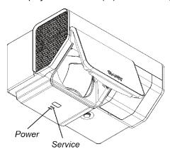
• The ECP's **Power** button (see *Using the Extended Control Panel (ECP)* on page 24) also functions as a status light.
