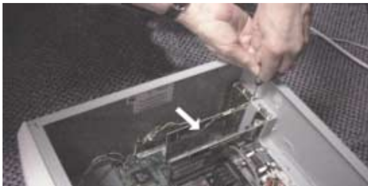
Inserting your Modem into a PCI Slot
