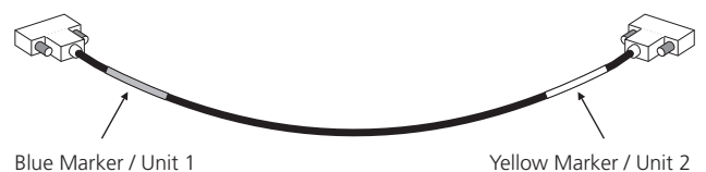
Figure 1 The Interconnect Cable
