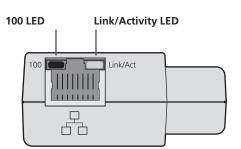
The following tables describes how to interpret the LED signal. The 100 signal varies depending on the speed of the device that is connected to the USB Network Ethernet Adapter. If you detect a problem, contact 3Com technical support.
