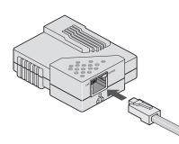
Insert the other end of the Ethernet cable into an available Ethernet port on a broadband modem, hub, home gateway, or other Ethernet Internet device.
