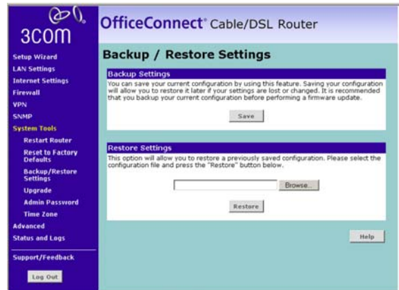
Figure 51 Backup/Restore Settings Screen
