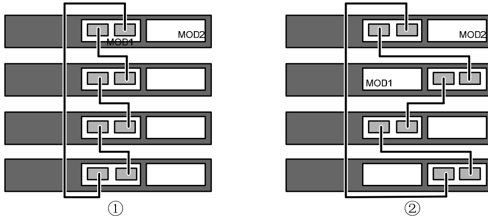
Figure 3-27 Cable connections in an IRF in the non-aggregate mode with 2-port interface modules
