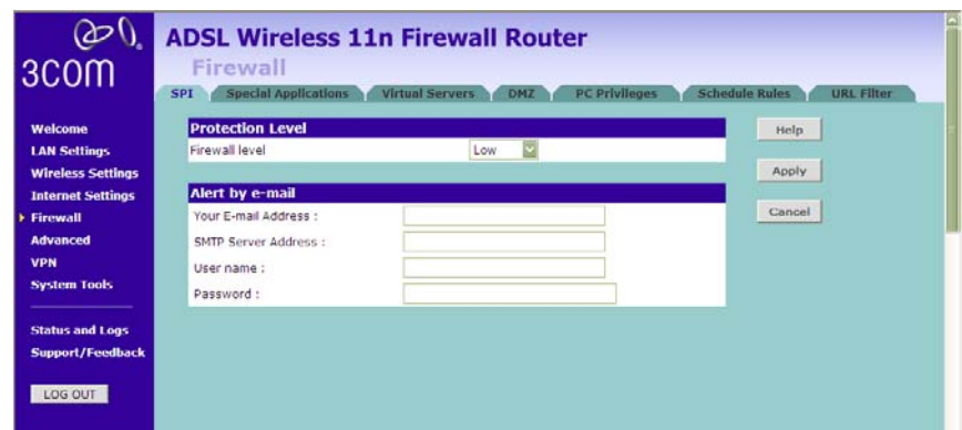
Figure 69 Low and Medium Level Firewall Protection Screen
