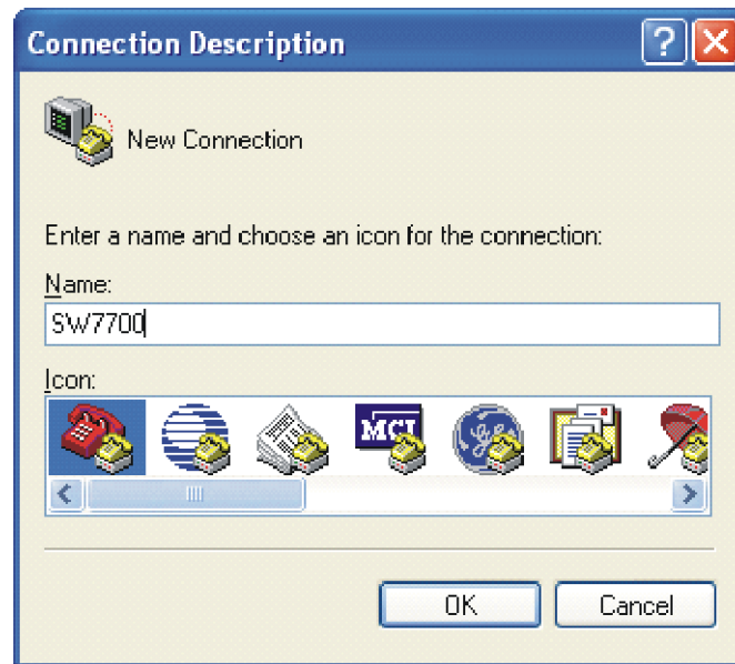
Figure 2 Set Up the New Connection
