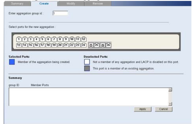
Figure 43 Link Aggregation Create Screen
