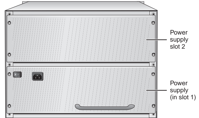
Figure 2 Switch 4007 Chassis Rear View
