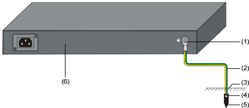
Figure 3-7 Ground the switch by burying the grounding conductor into the earth
