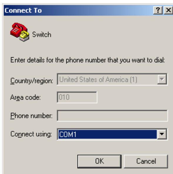
Figure 4-4 Set the serial port used by the HyperTerminal connection
