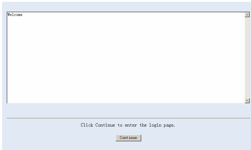
Figure 4-5 Banner page displayed when a user logs in to the switching engine through Web
