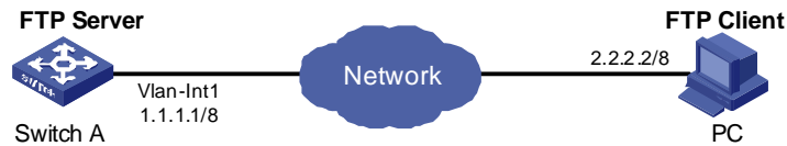
Figure 1-3 Network diagram for FTP configurations: the device operating as an FTP server
