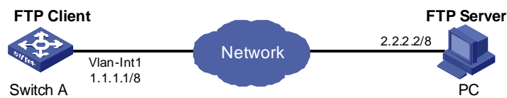
Figure 1-5 Network diagram for FTP configurations: the device operating as an FTP client
