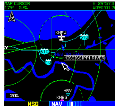
Figure 7-41 Activate Panning Function
