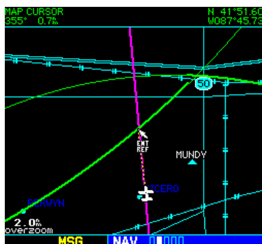
Figure 3-22 Using Pointer to Measure Distance and Bearing
