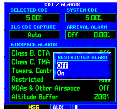
Figure 10-31 Restricted Alarm Window
