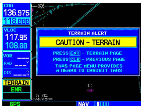
Figure 13-3 Caution Alert Pop-up
