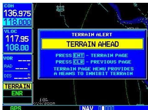
Figure 12-4 TERRAIN Caution Pop-up (Flashing)
