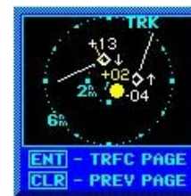
Figure 14-13 Traffic Warning Window
