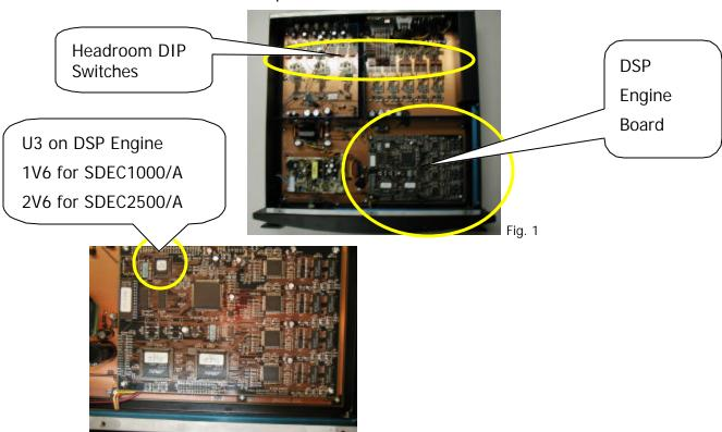
3. Locate U3 on the DSP Engine Board (see Fig.2).
