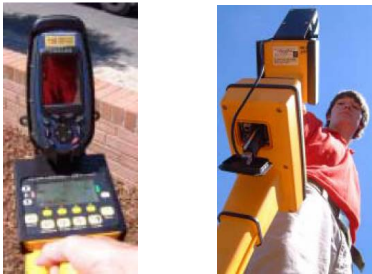
Figure 13. Thales™ MobileMapper™ mounted on 3M™ Dynatel™ Locator
