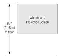
2. The Digital Media System 800 Series can project an image size between 50" (1,270 mm) and 85" (2,160 mm), measured diagonally (when mounted on the same plane as the projected surface). Measure the whiteboard if necessary to determine the size image you intend to use.
