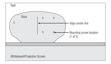
5. Determine the appropriate anchor to use with your wall type. Install five anchors at the marked locations. Install, but do not tighten, five mounting screws.
