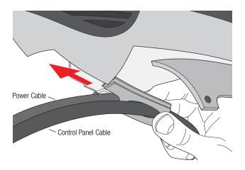
12. Connect the control panel and power cables as shown.
