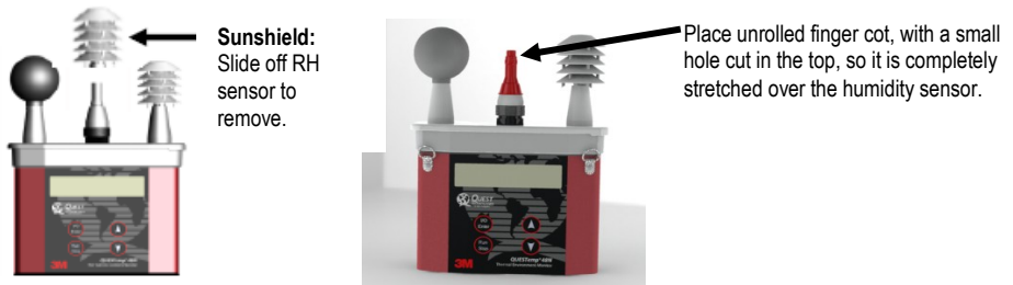
Figure 1-26: Sunshield & placement of finger cot prior to RH alignment
