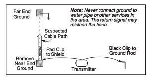
Make sure the Transmitter is off. Plug the direct connect cable into the front panel jack. Connect the Black clip to the ground rod. Place the ground rod in the earth perpendicular to the suspected cable path. If necessary, extend the black lead with the Ground Extension Cable. Remove the ground bonding and attach the Red clip to the shield.
