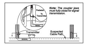
Connect the Dyna-Coupler to the Transmitter front panel jack using the coupler cable.
