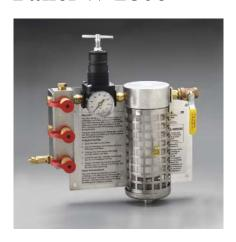
This panel is designed to filter and regulate air being delivered to the supplied air respirator. It has a maximum capacity of 50 cfm at 105 psig. This is an economical system that provides single step filtration. It is designed to be permanently mounted to the wall. It provides a maximum of 50 cfm to 3-5 outlets.
