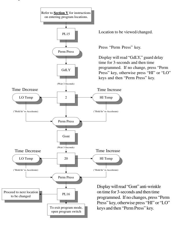
Summary: Guard delay time is programmable from 1 to 9 minutes. Guard on time is programmable from 1 to 99-seconds.
