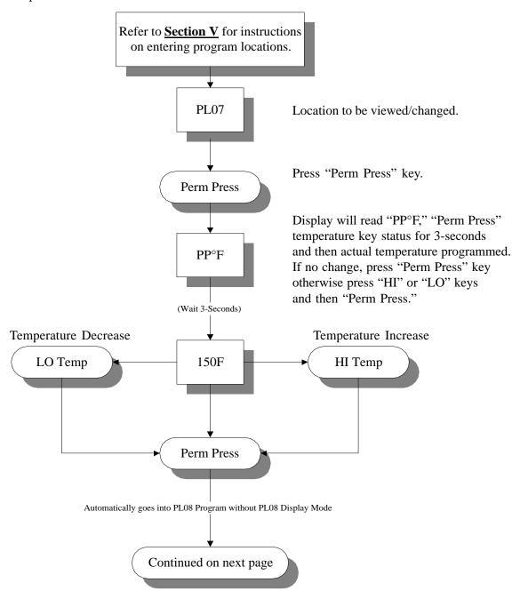
Summary: Perm Press Temp is programmable from a minimum of 100° F to a maximum of 190° F in ten-degree increments or from a minimum of 38° C to a maximum of 88° C in five-degree increments. For the **AD-26 and AD-295** any three (3) of the selections (HI/LO/PP) are programmable from a minimum of 100° F to a maximum of 170° F in ten-degree increments or from a minimum of 38° C to a maximum of 77° C in five-degree increments.
