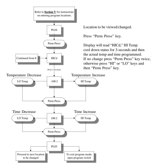
Summary: Cool down temperature is programmable from a minimum of 70° F to a maximum of 190° F in ten degree increments or from a minimum of 21° C to a maximum of 88° C in five-degree increments.
