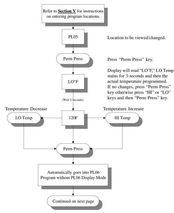
Summary: LO Temp is programmable from a minimum of 100° F to a maximum of 190° F in ten-degree increments or from a minimum of 38° C to a maximum of 88° C in five-degree increments.
