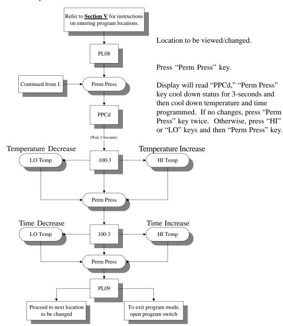
Summary: Cool down temperature is programmable from a minimum of 70° F to a maximum of 190° F in ten-degree increments or from a minimum 21° C to a maximum of 88° C in five-degree increments. For the **AD-26 and AD-295** any three (3) of the selections (HI/LO/PP) are programmable from a minimum of 100° F to a maximum of 170° F in ten-degree increments or from a minimum of 38° C to a maximum of 77° C in five-degree increments.
