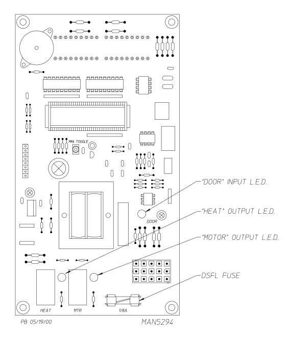
There are three (3) L.E.D. indicators ("red" lights) located at the lower back side area of the microprocessor controller (computer) which are identified/labeled as "DOOR," "HEAT," and "MTR" (motor). These L.E.D.s indicate that the outputs of the microprocessor controller (computer), or in the case of the door switch, the inputs are functioning.
