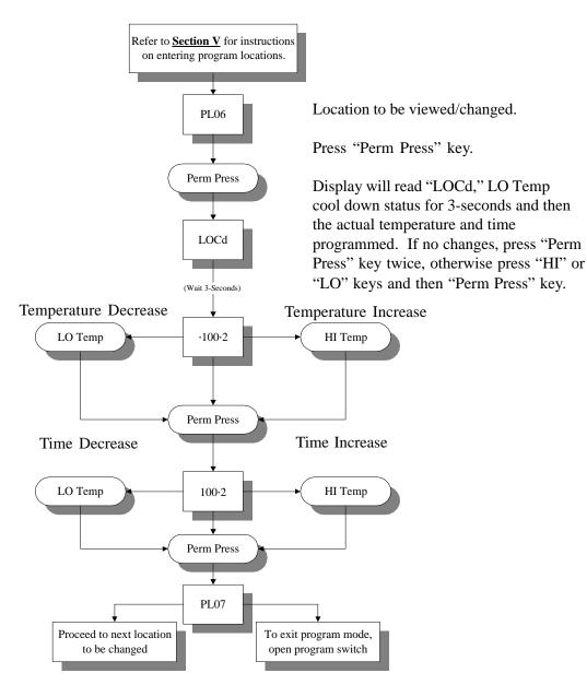
Summary: Cool down temperature is programmable from a minimum of 70° F to a maximum of 190° F in ten degree increments or from a minimum 21° C to a maximum of 88° C in five-degree increments.
