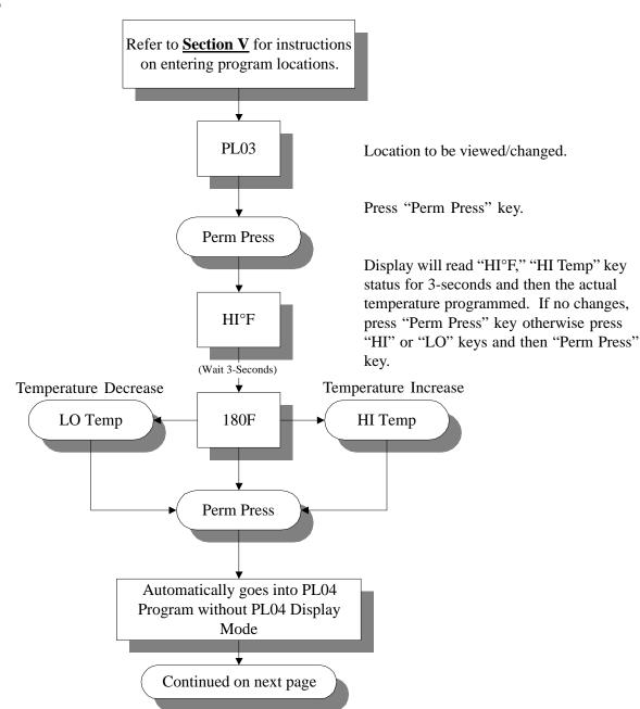
Summary: HI Temp is programmable from a minimum of 100° F to a maximum of 190° F in ten-degree increments or from a minimum of 38° C to a maximum of 88° C in five-degree increments.
