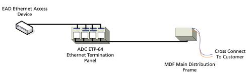
The ADC ETP-64 Ethernet termination panel accepts the 50 pin AMP type connectors from the Ethernet access device (EAD) and transitions to LSA-PLUS NT circuit terminations that are cabled to MDF and terminated on blocks that support cross connecting to individual circuit assignments.
