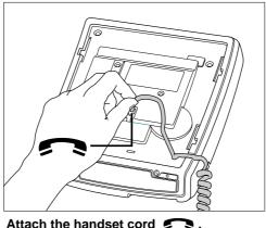
Attach one end of the handset cord to the handset and the other end to the handset jack.
