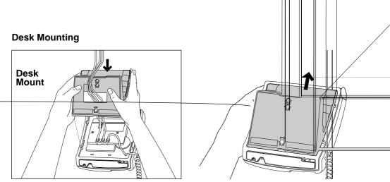
Lower the stand into the slots on the base of the telephone, as shown in the desk mount illustration above. Slide the stand back until it clicks into the locked position. The excess line cord fits into the stand of the telephone.
