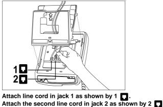
Attach one end of the line cord to jack number 1 and the other end to the wall jack. Attach the second line cord to jack number 2 and the other end to the wall jack. Both line cords are supplied with the telephone.
