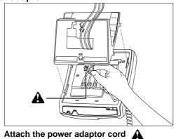
Attach the power adaptor to the base of the telephone, where the warning symbol is marked. Then connect the power adaptor into the closest electrical outlet.
