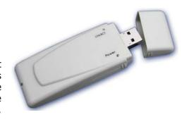
This device is the perfect solution for your wireless network applications based on the IEEE 802.11b standard that offers a data rate up to 11Mbps in a wireless LAN environment. It is a high-speed wireless network card that plugs into your notebook or desktop PC and accesses to the LAN or peer-to-peer networking easily without wires or cables. Whether you're at your desk or in the boardroom, it allows you to share printers, files, and other network resources.
