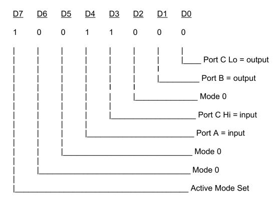
This corresponds to 98 hex. If the card base address is 2D0 hex, use the BASIC OUT command to write to the control register as follows:
