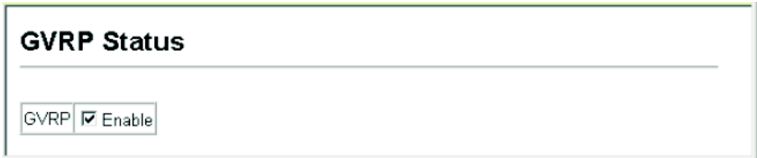
Figure 3-74 Globally Enabling GVRP
