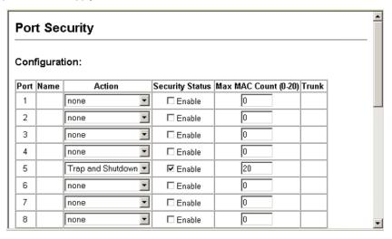
**CLI** – This example sets the command mode to Port 5, sets the port security action to send a trap and disable the port, and then enables port security for the switch.
