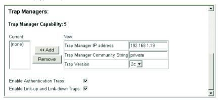
**CLI** – This example adds a trap manager and enables both authentication and link-up, link-down traps.
