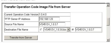
If you download to a new destination file, then select the file from the drop-down box for the operation code used at startup, and click Apply Changes. To start the new firmware, reboot the system via the System/Reset menu.
