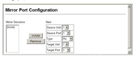
**CLI** – Use the interface command to select the monitor port, then use the port monitor command to specify the source port. Note that default mirroring under the CLI is for both received and transmitted packets.
