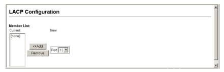
**CLI** – The following example enables LACP for ports 13 and 14. Just connect these ports to LACP-enabled trunk ports on another switch to form a trunk.
