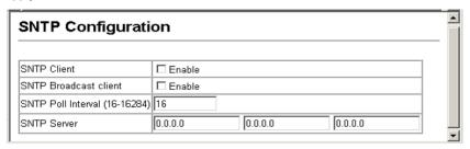
**CLI** – This example configures the switch to operate as an SNTP client and as an SNTP broadcast client.
