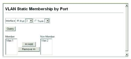
**CLI** – This example adds Port 3 to VLAN 1 as a tagged port, and removes Port 3 from VLAN 2.
