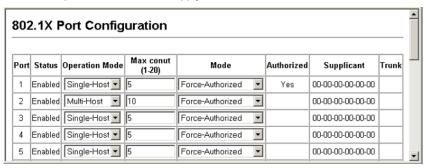
**CLI** – This example sets the authentication mode to enable 802.1x on port 2, and allows up to ten clients to connect to this port.
