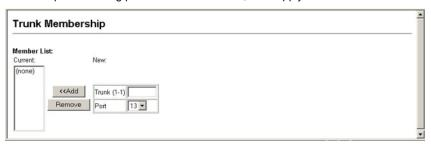
**CLI** – This example creates trunk 2 with ports 13 and 14. Just connect these ports to two static trunk ports on another switch to form a trunk.
