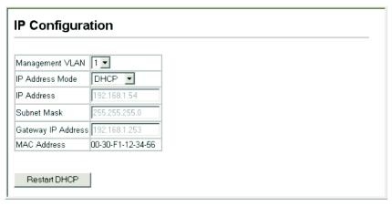
**Note:** If you lose your management connection, use a console connection and enter "show ip interface" to determine the new switch address.
