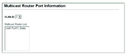
**CLI** – This example shows that Port 11 has been statically configured as a port attached to a multicast router.
