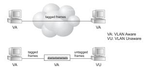
**VLAN Classification** – When the switch receives a frame, it classifies the frame in one of two ways. If the frame is untagged, the switch assigns the frame to an associated VLAN (based on the default VLAN ID of the receiving port). But if the frame is tagged, the switch uses the tagged VLAN ID to identify the port broadcast domain of the frame.
