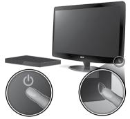
• On the Acer 3D monitor, press Input to set the HDMI™ source.
