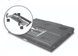
Replace the memory compartment door, and fasten the screw.
