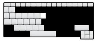
To use the embedded numeric keys, toggle the Num Lk on by pressing the Fn + F9 keys simultaneously.
