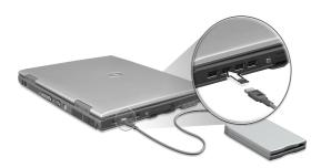
USB is plug and play, which means that you can connect and start using a USB device without having to restart your computer. You can also disconnect the device at any time.
