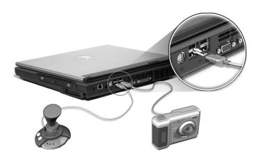
USB is plug and play, which means that you can connect and start using a USB device without having to restart your computer. You can also disconnect the device at any time.
