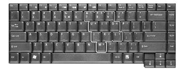
To use the embedded numeric keys, toggle the Num Lk on by pressing the Fn + F11 keys simultaneously.
