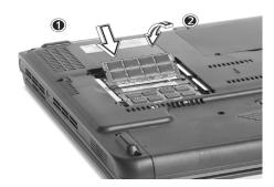
4 Replace the memory compartment door, and fasten the screw.
