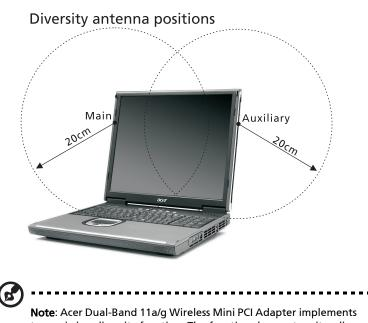
**Note**: Acer Dual-Band 11a/g Wireless Mini PCI Adapter implements transmission diversity function. The function does not emit radio frequencies simultaneously from both antennas. One of the antennas is selected automatically or manually (by users) to have good quality of radiocommunication.
