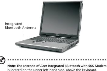
**Note**: The antenna of Acer Integrated Bluetooth with 56K Modem is located on the upper left-hand side, above the keyboard. Transmitted energy from the Bluetooth device is very low compared to other RF devices. Therefore, a 20 cm separation from the Bluetooth antenna is not required.
