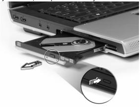
When the power is off, you can eject the drive tray using the emergency eject hole.
