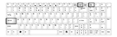
The computer features three lock keys, each with its own status indicator light.
