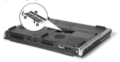
4 Replace the memory compartment cover, and fasten the screw. The computer automatically detects the new module and reconfigures the system memory.
