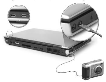
USB is plug and play, which means you can connect and start using a USB device without having to restart your computer. You can also disconnect the device at any time.
