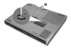
3 Insert the memory module diagonally in the slot (a), and then press down gently until it clicks in place (b).
