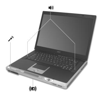
The built in sub-woofer provides tight and precise bass performance for low frequency audio.
