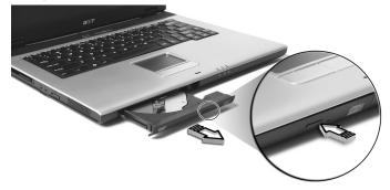
When the power is off, you can eject the drive tray using the emergency eject hole. See page 48.
