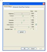
**Device Settings** allows you to change the camera brightness, contrast, hue, saturation, sharpness, etc.
