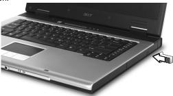
When the power is off, you can eject the drive tray by using the emergency eject hole.
