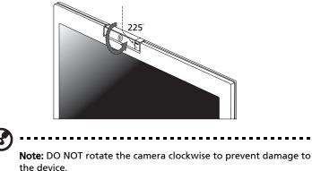
For your convenience, the camera snaps to 45 degrees to match the position of your face in front or at the back of the LCD panel.
